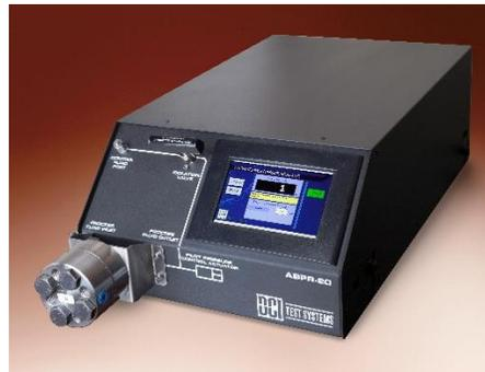
The ABPR has multiple operating modes. One useful mode is the process pressure control and allows the user to connect an external pressure transducer to the APBR in the process line and control to that signal.
