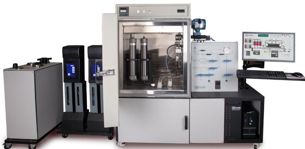
HIGH PRESSURE HIGH TEMPERATURE FOAM RHEOMETER (PICTURED WITH BOOSTER CART)
