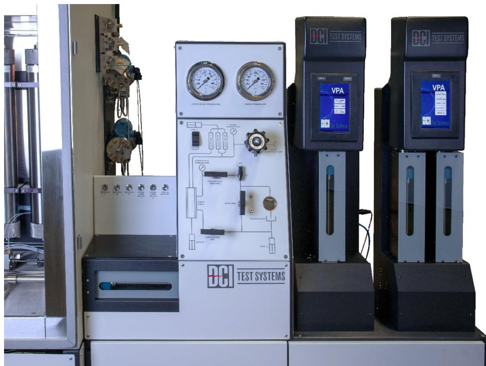
VPA SYRINGE PUMPS INTEGRATED INTO CORE FLOOD SYSTEM
