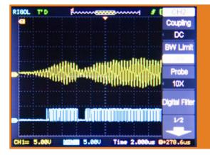
Separator operation can be understood by the reflected wave from both the meniscus and target on a oscilloscope.
