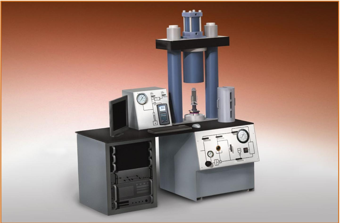
The Integrated Rock Mechanics Test System was developed by DCI in response to a need for a compact triaxial rock mechanics test systems suitable for performing routine triaxial tests on plug-size rock samples. Integrated into a single desk-size test system, the systems include:
